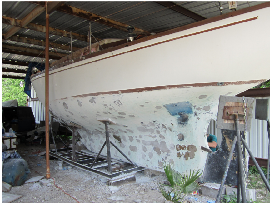
Side view showing repaired blisters
